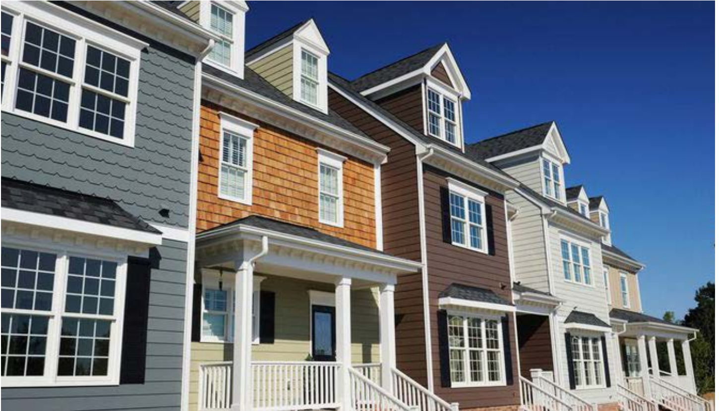
Figure 33. Articulation can break up the massing of housing blocks and provide visual interest (Realtor.com).
