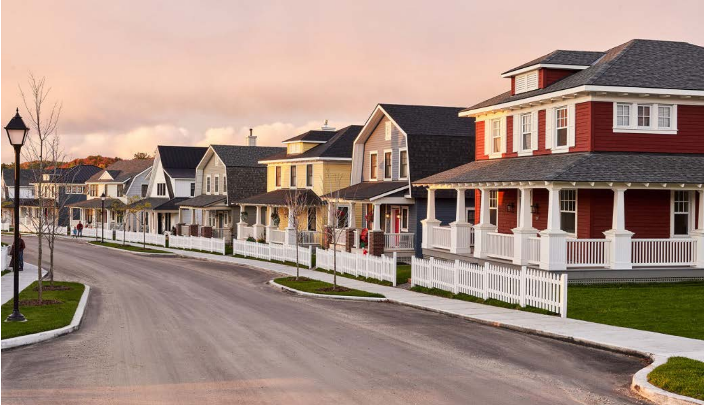
Local roads should have as narrow right-of-ways as practical to slow traffic and provide space for pedestrian circulation and street trees (Landlab Inc).
