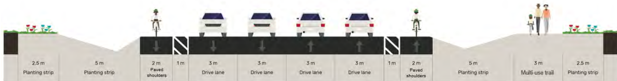
Exhibit 5-22: Typical Midblock Cross Section, 36m Type B Arterial, Four-Lane Rural with Class I trail (In-Boulevard Multi-use Trail) and On-Road Cycling Lanes (Paved Shoulders)
