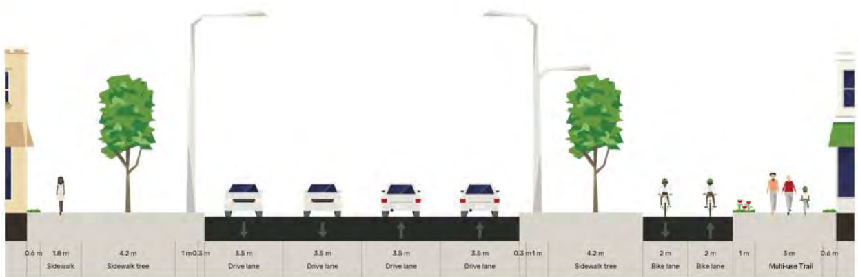
Exhibit 5-25. Typical Midblock Cross Section, 36m Type B Arterial, Four-Lane Urban with Class I trail (In-Boulevard Multi-use Trail) and On-Road Cycling Lanes (Bike Lanes)
