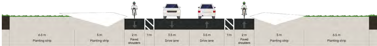
Exhibit 5-21: Typical Midblock Cross Section, 36m Type B Arterial, Two-Lane Rural with On-Road Cycling Lanes (Paved Shoulders)
