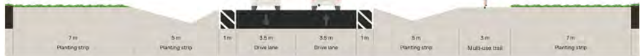
Exhibit 5-20. Typical Midblock Cross Section, 36m Type B Arterial, Two-Lane Rural with Class I Trail (In-Boulevard Multi-use Trail)
