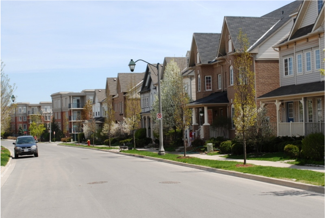
Figure 12. Local roads should have as narrow right-of-ways as practical to slow traffic and provide space for pedestrian circulation and street trees (Brook McIlroy).
