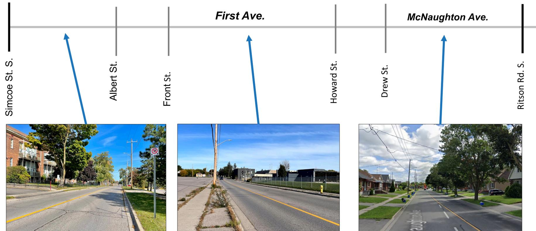
The existing corridor of First Ave./McNaughton Ave. has two vehicle lanes with sidewalks on both sides (sidewalks are approximately 1.3 to 1.5 metre in width) separated by either a grass or concrete buffer from the road. The schematic and pictures above illustrate the present configuration and road cross sections.
