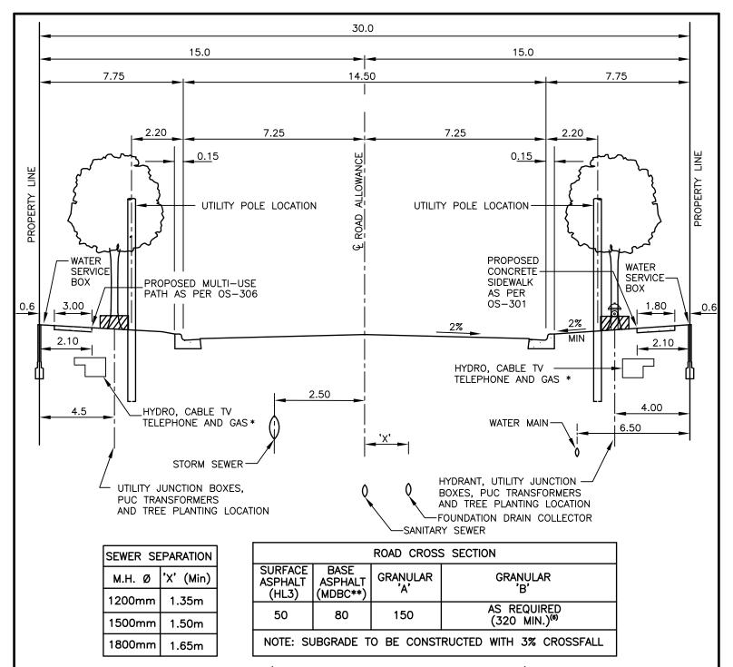
NOTES: 1. FOR TWO PIPE SYSTEM (TYPE II STORM SEWER AND SANITARY SEWER) REFER TO DRAWING OS-207.
